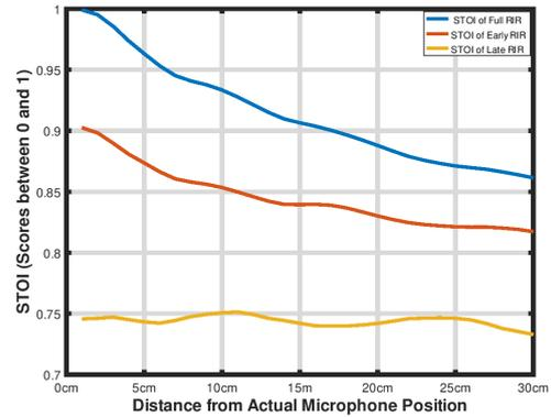
Figure 5: STOI variation with varying microphone positions.
