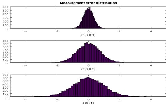
Figure 1: Microphone position error ( $\epsilon_x, \epsilon_y, \epsilon_z$ ) for  $\sigma^2 = 0.1, 0.5, 1$ .
