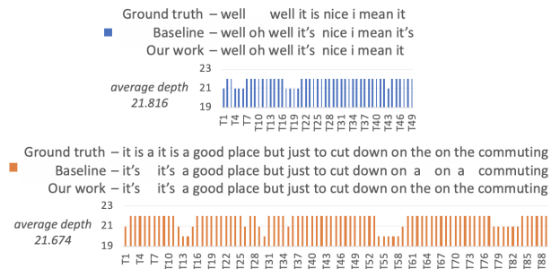
Figure 3: Number of encoder layers required N_i in Eq. 3 for each time step i and average encoder depth of two randomly sampled speech utterances from Switchboard test dataset.
