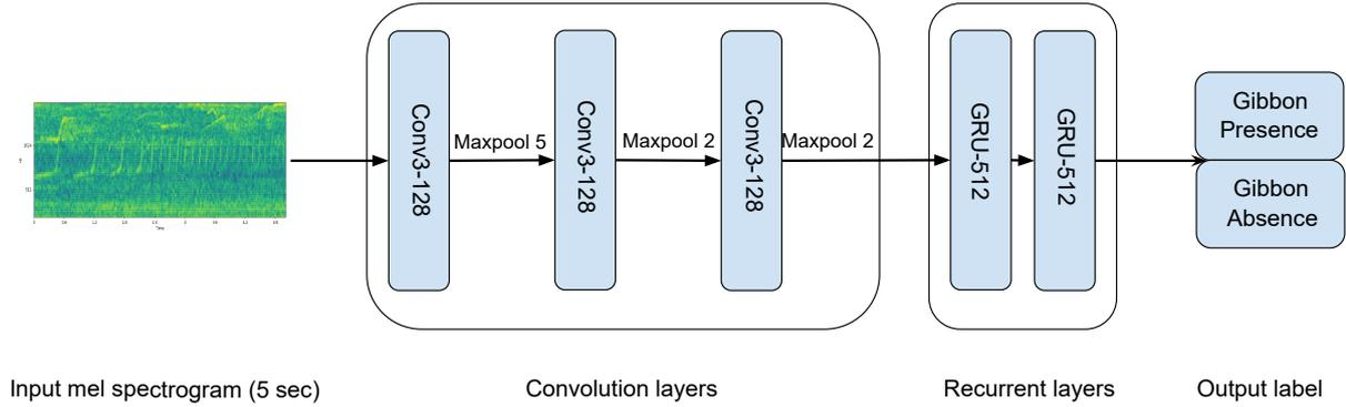
Figure 2: *Proposed deep neural network architecture. The input representation is passed through a convolution neural network before passing to a recurrent neural network with gated recurrent units for the final prediction.*
